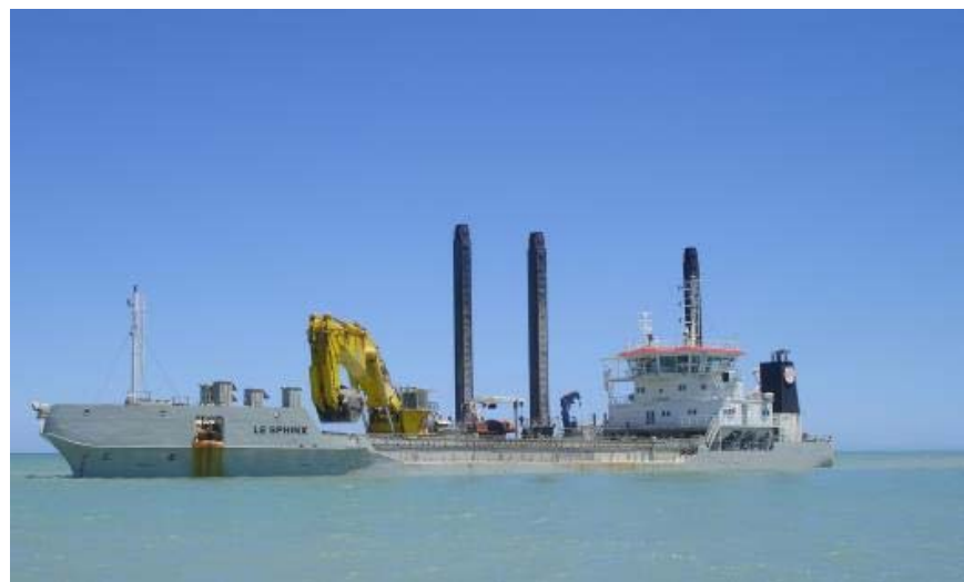
Figura 8-8 : “Bachoe Dredger” 'Mimar Sinan' con “Split Hopper Barge”
