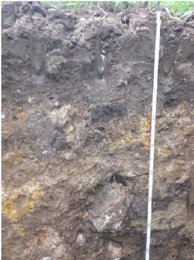
Fot. 3 Profilo AV-DE-A3-ST-05-GR2-01 dettaglio Orizzonte Ap (0-35 cm), AB (35-53 cm), BA (53-65 cm)
