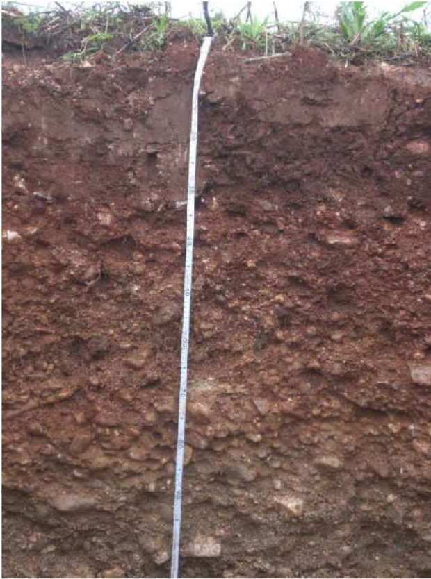
Fot. 3 Profilo AV-CA-A1-ST-07-GR2-04 dettaglio Orizzonte Ap (0-30cm), B1 (30-45cm) e B2 (45-70cm)
